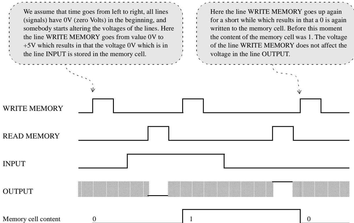
**Figure 3-3.** Writing and reading a single-bit memory cell.
